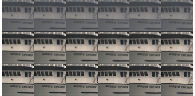
Fig. 3. Zoom-in snapshots of the sequence “acoustic explorer”. Top: input video sequence. Middle: contrast enhancement using gray-level grouping [13]. Bottom: applying deconvtv to the results of the middle row.
