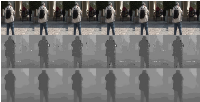
Fig. 2. Disparity map estimation result of “Old Timers” sequence. Top row: stereo video input (left view). Middle row: initial map estimation using loopy belief propagation [10]. Bottom row: result of applying deconvtv to the middle row. Parameters are \mu = 1 , (\beta_x, \beta_y, \beta_t) = (1, 1, 2.5) .
